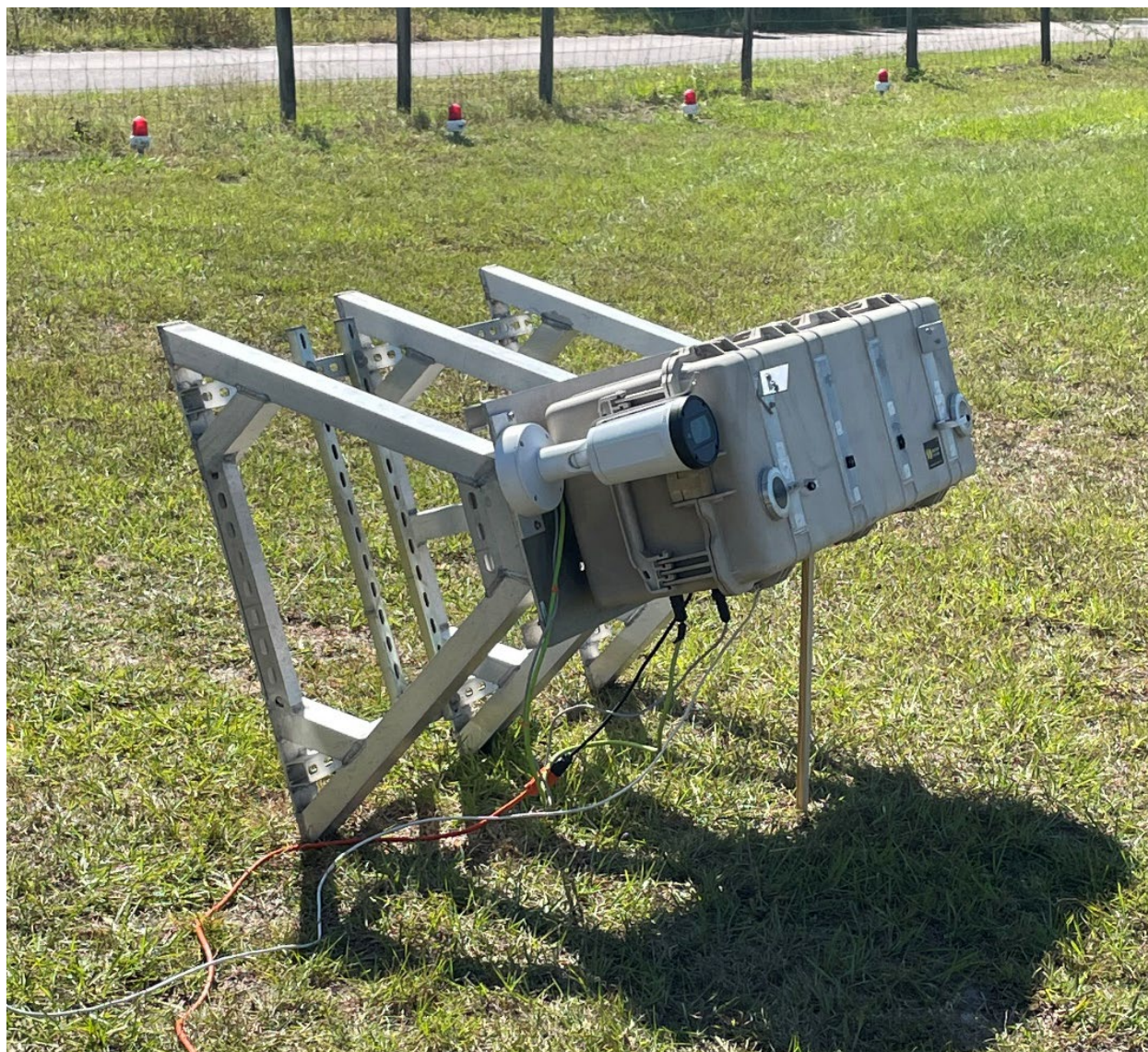
Figure B-2. ATOM system tilted to 22 degrees to accommodate longer distance testing otherwise restricted by the FAA 400-ft drone flight height restriction.
